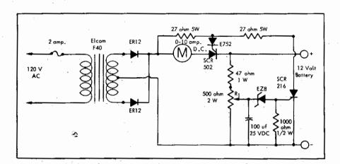
This battery charger will charge the battery at maximum possible rate until fully charged and then shut itself off. It will start itself when the battery becomes discharged and repeat the cycle.
